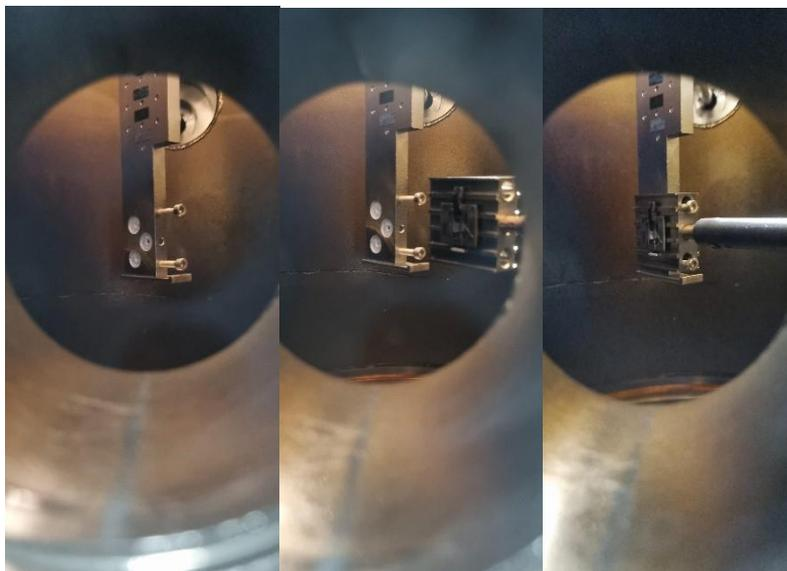
8. Slowly unscrew the transfer bar ensuring that the holder remains fully attached to the manipulator (guiding screws head clearly visible);
