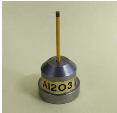
Figure 11 - Capillary in the PIN and ready to start the experiment
