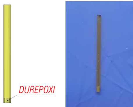
Figure 7 - Capillary with one extremity sealed
