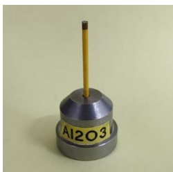
Figure 7 - Capillary in the PIN
