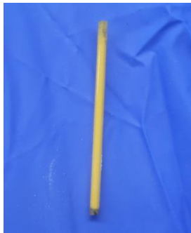
Figure 4 - Capillary filled with sample
