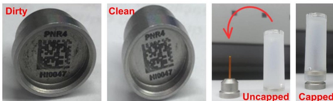
Figure 3 – Clean the PIN DataMatrix with isopropyl alcohol. DO NOT use acetone. Place the protective cap for transportation.
