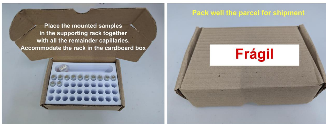
Figure 4 - Example showing how to prepare a parcel to ship samples back to Sirius after preparation and registration.
